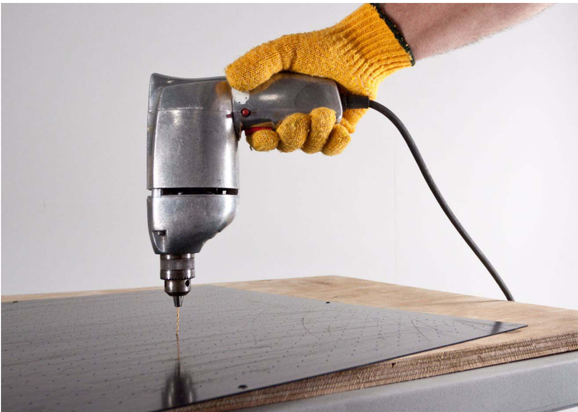
Figure 23 Drilling holes through the black plastic, smooth side up. Note that scrap wood is placed underneath.
