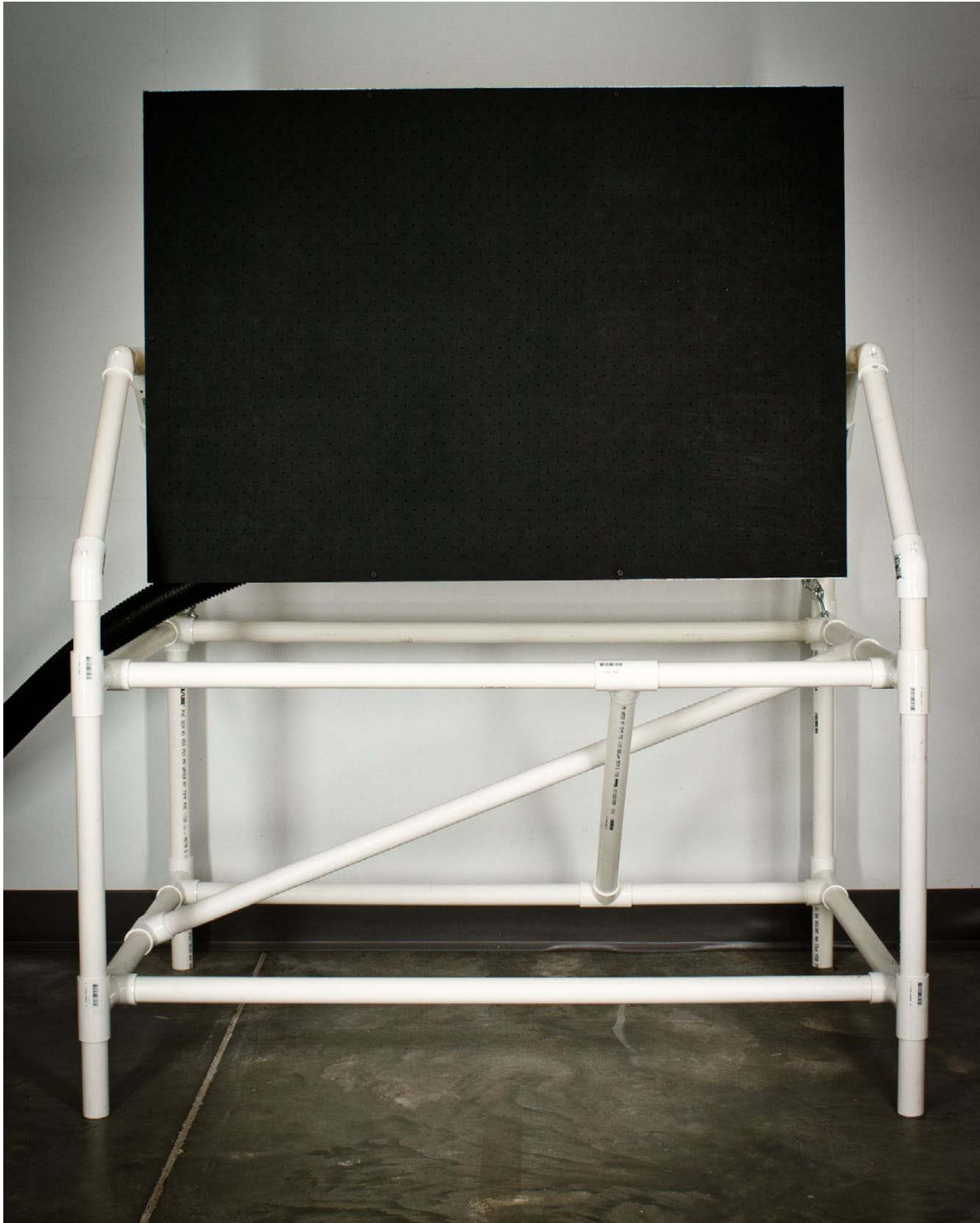
Figure 1 The completed vacuum table as seen from the front, with the top vertical.
