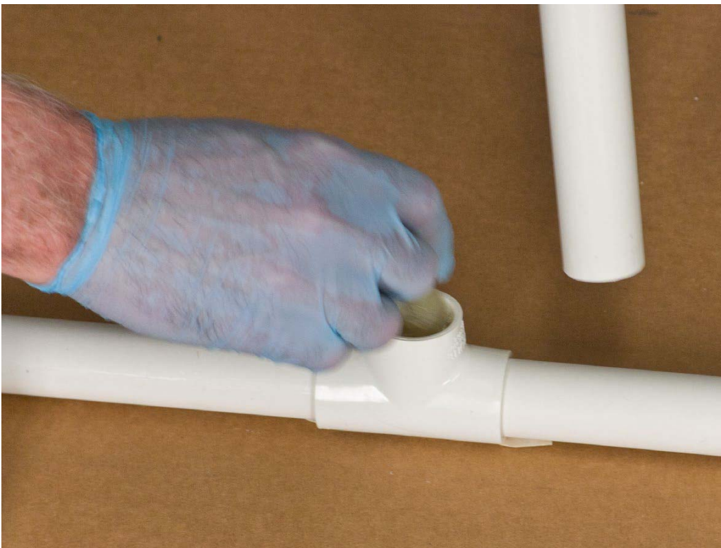
Figure 49 Wear gloves when gluing. Have adequate ventilation. Wear safety glasses. Be careful with PVC cement.
