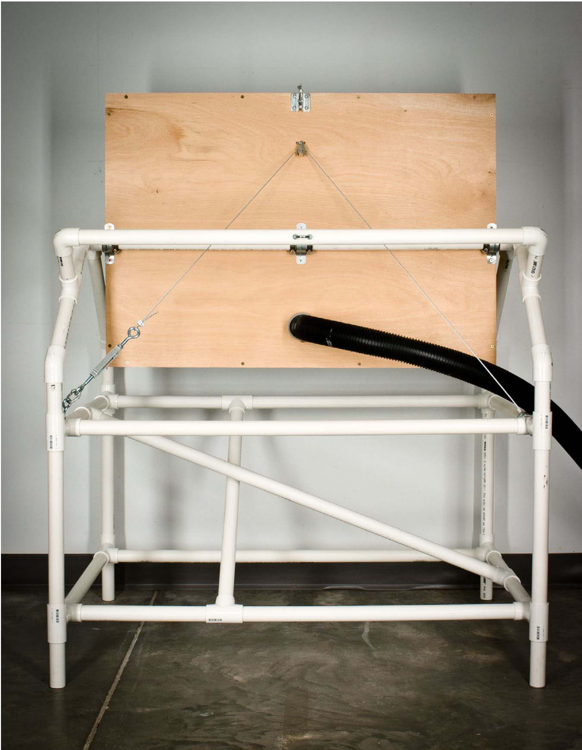
Figure 2 The completed vacuum table as seen from the rear, with the top vertical.
