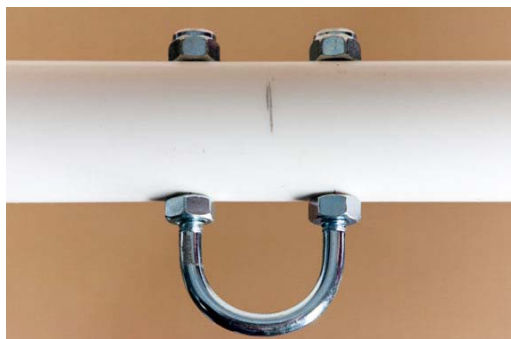
Figure 56: U-Bolt in place.
