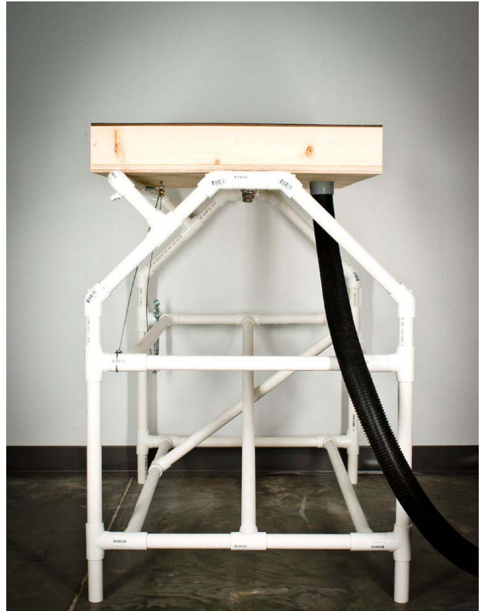
Figure 7 The completed vacuum table, opposite side view, with the top horizontal.
