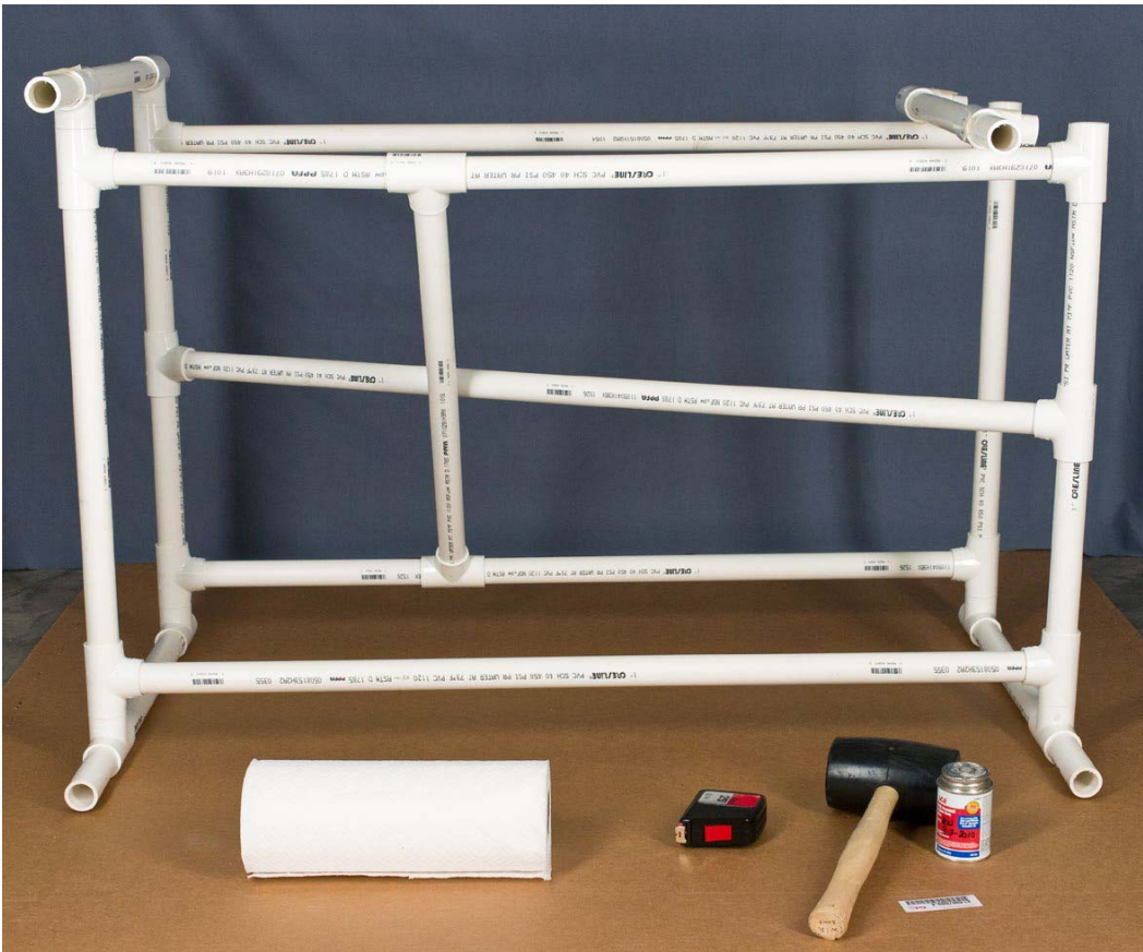
Figure 48 Pull apart one section. Have supplies ready, in preparation for gluing.
