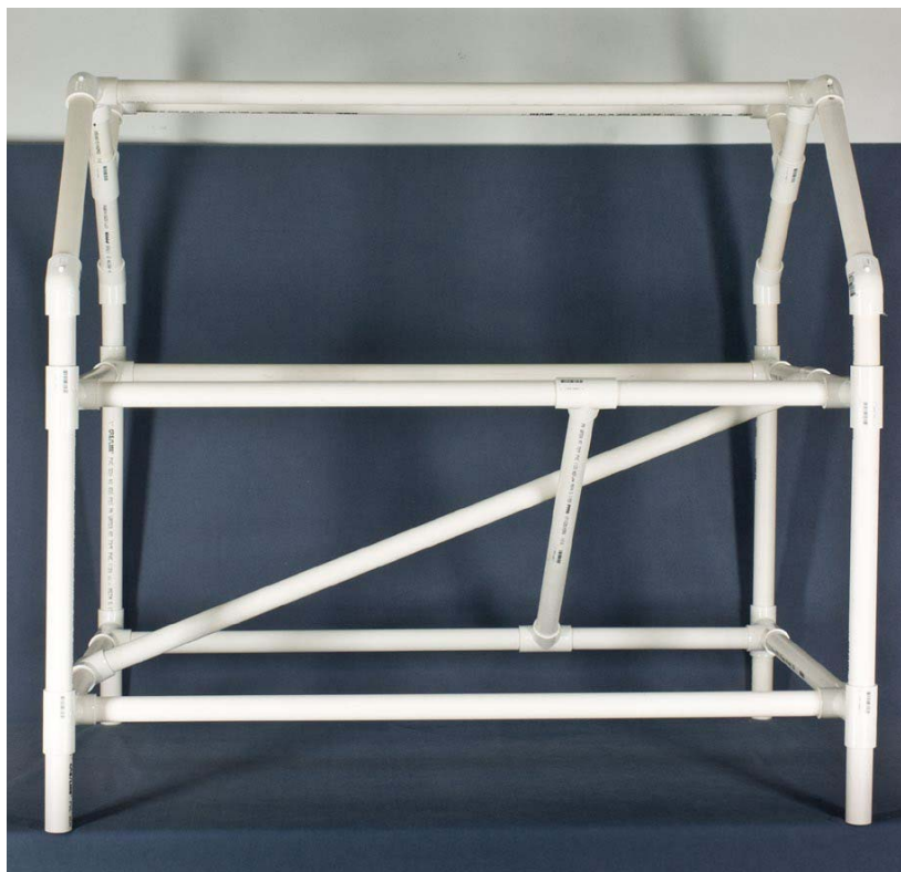
Figure 46 Completed base frame assembly, rear view. (Not yet glued.)
